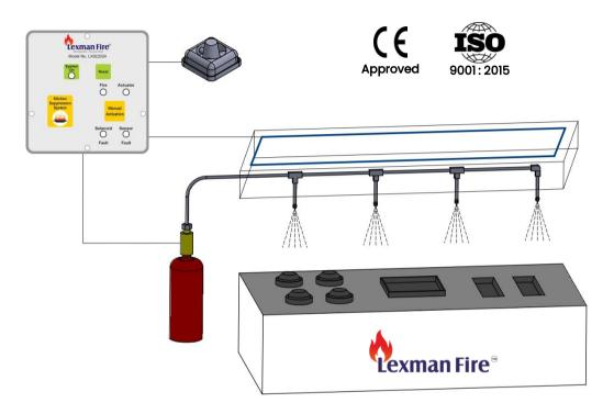
A Kitchen Fire Suppression System is a specialized fire protection solution designed to detect and extinguish fires in commercial and industrial kitchens. It provides automatic and manual fire suppression, ensuring the safety of kitchen staff, equipment, and property by quickly extinguishing fire caused by cooking oils, grease, and high-temperature appliances.
